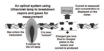
charge of the ionized gas and converts the signal into current. The current is then amplified and displayed on the meter as "ppm." Only a tiny fraction of the gas passing through the sensor is ionized; most passes through unchanged. RAE PIDs are not dependent on oxygen to make a measurement and PIDs fail safe. When the PID lamp fails to light the PID provides a "lamp" alarm so operators immediately know that it is not working.
