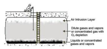
Before entering the confined space, take samples at several levels, and after entering, monitor the space continuously because conditions can change.
