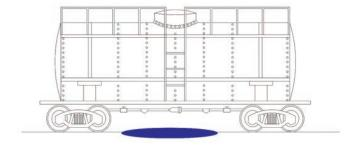
coming from condensation, not dripping benzene. The car had been loaded at 65°F and the high ambient temperature combined with relative humidity above 95% produced a puddle of water.
