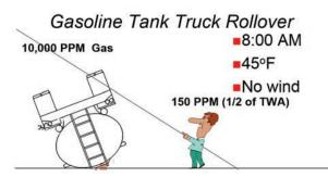
perimeter workers are often unprotected from changing conditions that may require movement of a perimeter away from the spill site. For many HazMat incidents, a PID allows those manning a perimeter line to adjust the line in response to changing conditions. PIDs can provide instantaneous alarms that warn perimeter workers when to retreat from an incident for everything from ammonia to xylene.
