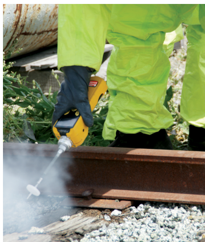
Workers can quickly measure VOCs and wirelessly transmit data
