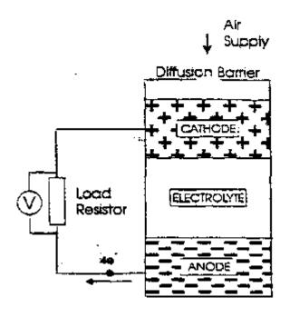
All oxygen sensors used are of the self-powered, diffusion limited, metal-air battery type comprising an anode, electrolyte and an air cathode as shown below.
