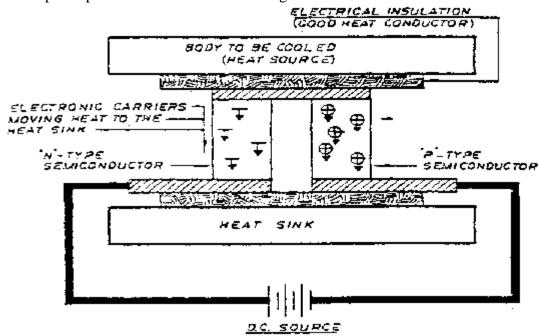
The basic function of a peltier element is the reversed thermoelectric effect that is used to measure temperatures with thermocouples. The so-called Seebeck effect causes two different metals, if welded together or held in close contact, to produce a particular voltage depending on the temperature.
